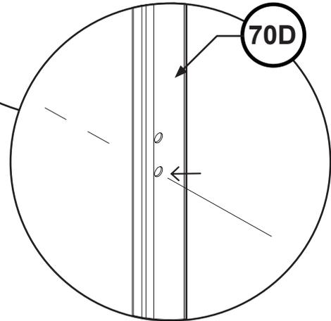
2. The four corner holes are to be drilled out into the top and bottom channels using the with the supplied 3mm drill bit and fastened from inside the panel using four FAST001 screws.
