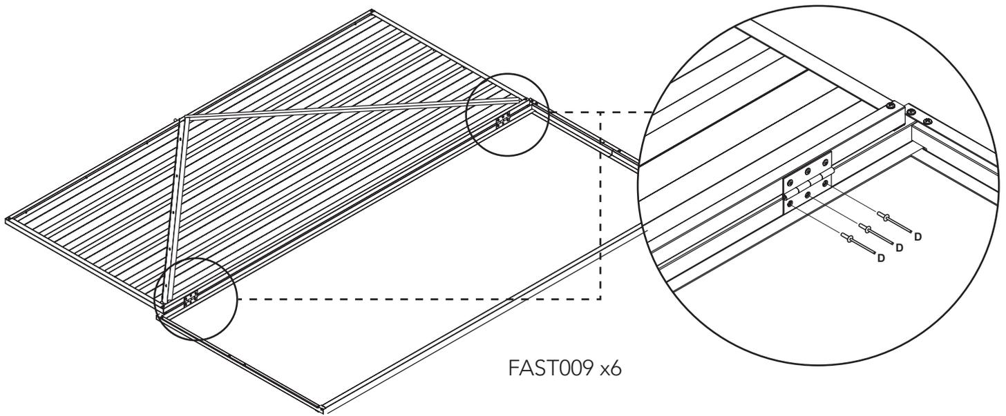
Lay the LEFT SIDE PANEL face up and lay the DOOR PANEL down in the open position on top as shown.
