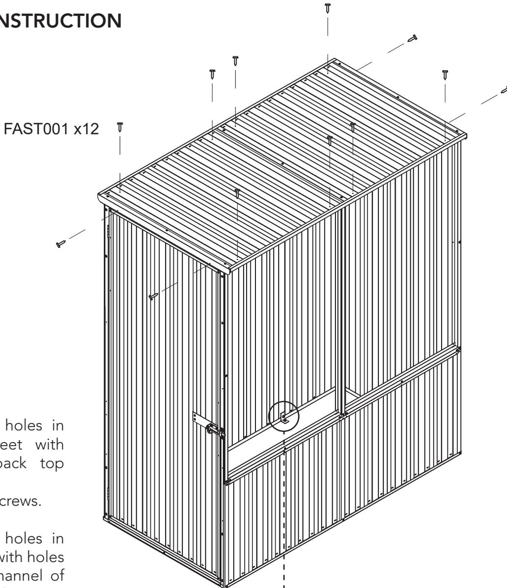
Line up the holes in the roof sheet with front and back top channels. Secure with screws.
